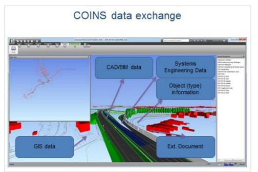
Figure 7: Open BIM-standard COINS for advanced data exchange
