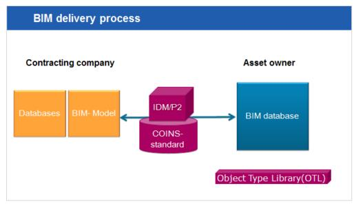
Figure 2: Dutch example of BIM-delivery process with the open information exchange standard COINS in Infrastructure
