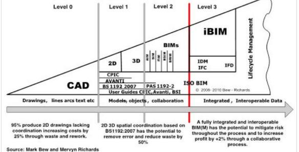
Figure 2: BIM Maturity model (UK BIM Taskforce)
